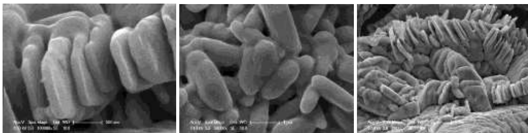
Figure 5. SEM images (left) x100000, (middle) x50000, (right) x20000 of CuO nanoparticles.
