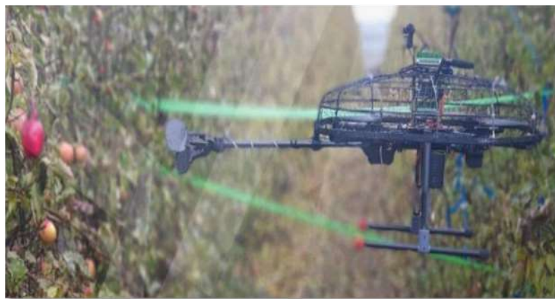
Figure 6. Autonomous harvesting vehicle (Güzey et al., 2020)
