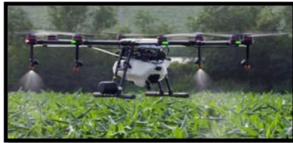
Figure 5. A drone spraying (Aydoğan, 2018)
