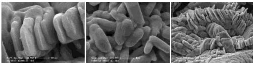
Figure 5. SEM images (left) \times 100000 , (middle) \times 50000 , (right) \times 20000 of CuO nanoparticles.
