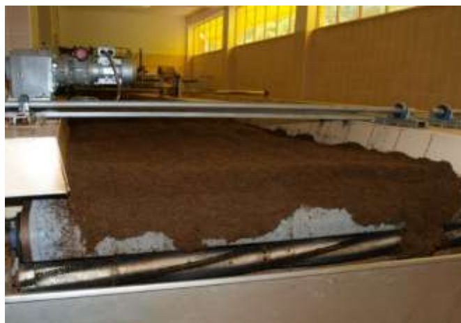
Figure 5. Oxidation Process of Tea Leaves
