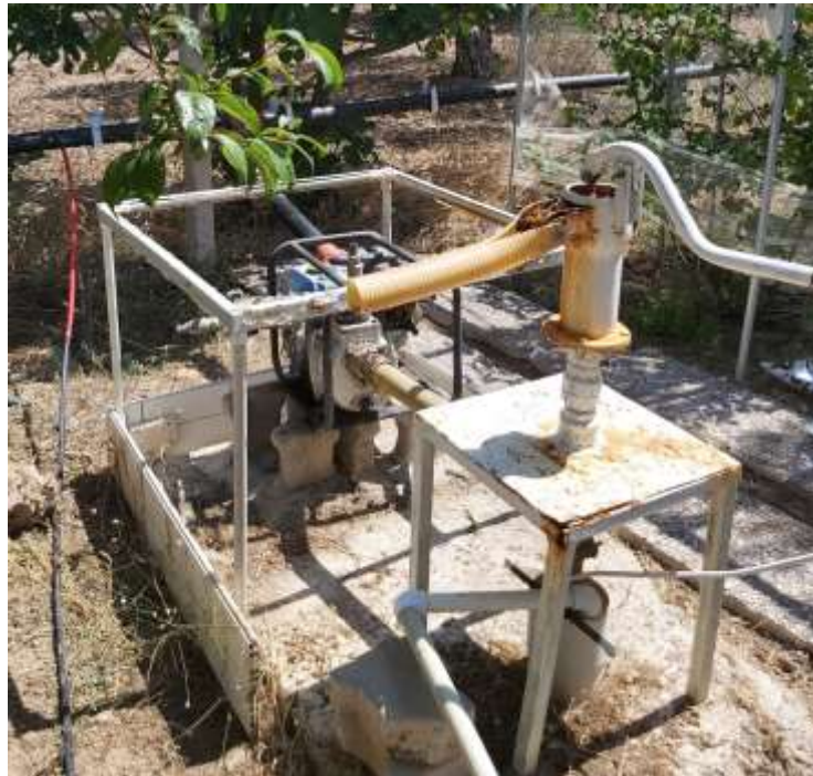
Figure 4. Schematic diagram of the gasoline-based water pumping system for drip irrigation
