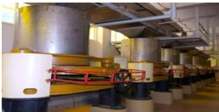
Figure 4. Rolling Process of Tea Leaves (Bellied Rolling)
