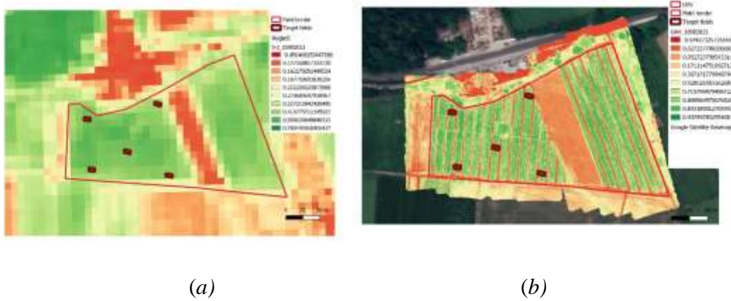
Figure 6. NDVI values: Sentinel-2 (a) and DJI Phanthom 4 Multispectral (b)
