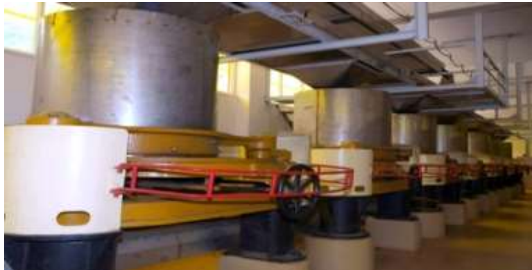
Figure 4. Rolling Process of Tea Leaves (Bellied Rolling)
