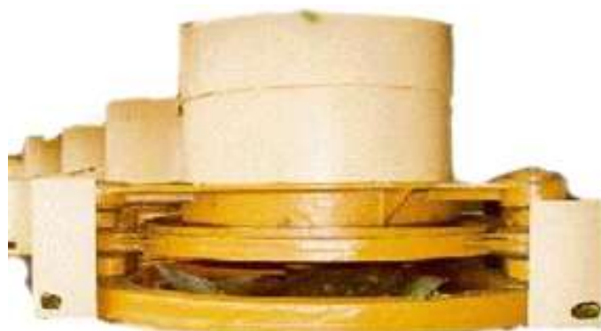
Figure 2. Rolling Process of Tea Leaves (Flat Rolling)
