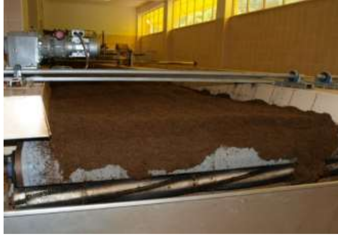
Figure 5. Oxidation Process of Tea Leaves
