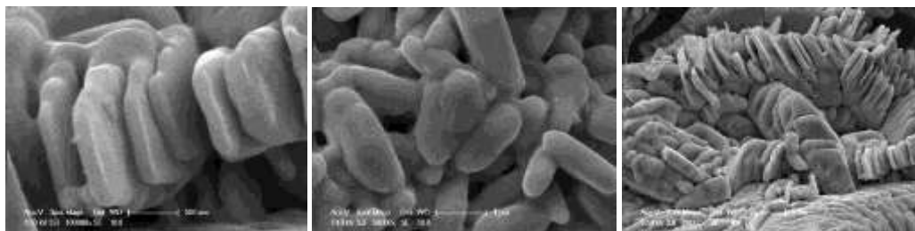
Figure 5. SEM images (left) x100000, (middle) x50000, (right) x20000 of CuO nanoparticles.
