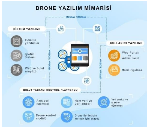
Figure 3. Drone software architecture template (Inan and Karci, 2021)
