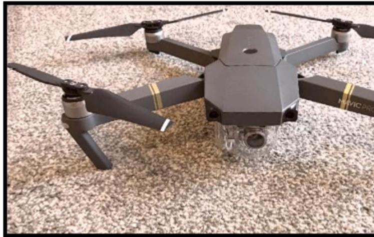
Figure 7. A drone DJI Mavic Pro used in animal census (Soares et al., 2021).
