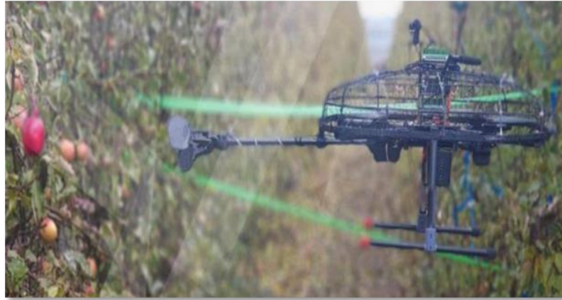
Figure 6. Autonomous harvesting vehicle (Güzey et al., 2020)
