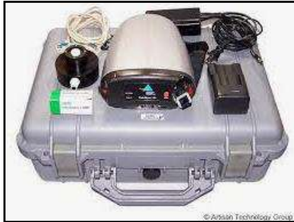
Figure 2. The portable hand held FieldSpec spectroradiometer (ASD Inc., USA)
