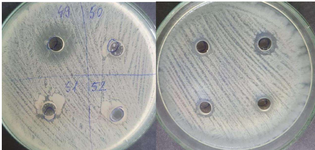
Figure 2. Agar well diffusion method for determining A) the antibacterial activity of Bacillus spp. from the soil samples against Bacillus subtilis ATCC 6633. B) the antibacterial activity of Bacillus spp. from the wastewater samples against Bacillus subtilis ATCC 6633.
