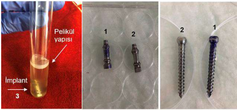
Figure 2. Biofilm structures on a dental implant. The crystal violet stained (purple) regions on the surface show the biofilm structures. 1: The implant surface tested with the biofilm reactor, 2: The implant surface tested with the batch system, 3: The implant surface in the batch system and the pellicle structure formed in the liquid-air interface.
