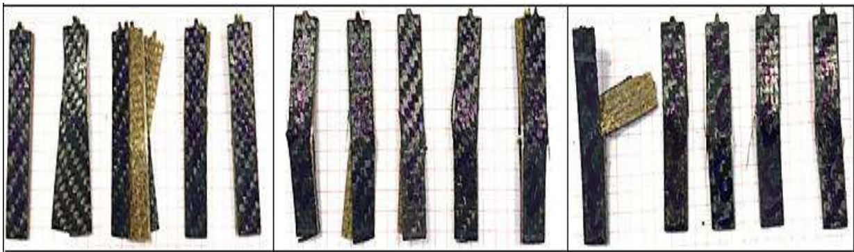
Figure 5. Post-test appearances of the Charpy Impact-tested samples of Jute Prepreg Composites
