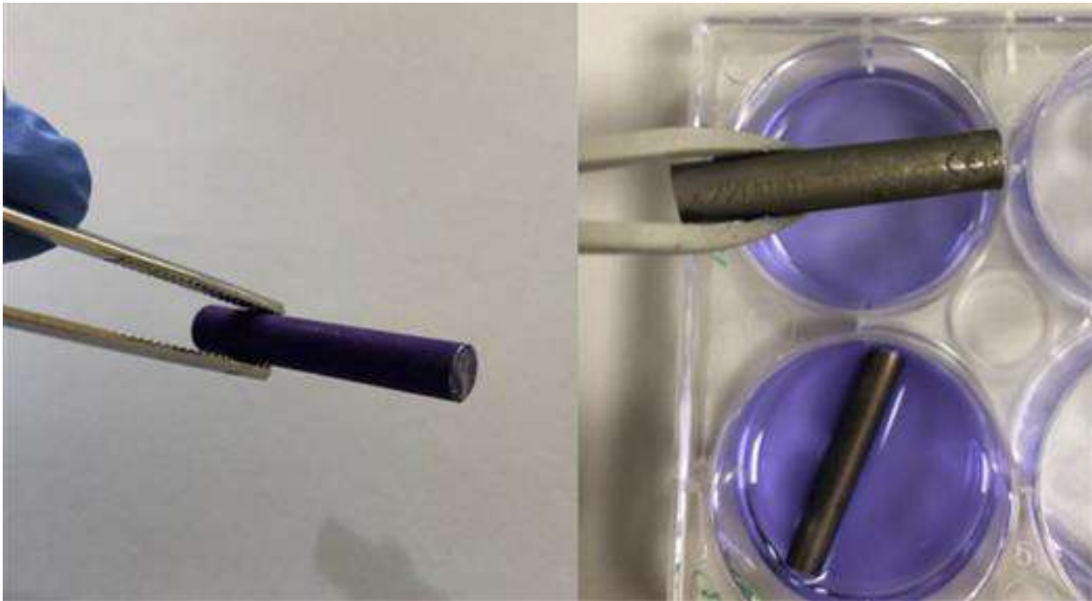
Figure 3. Biofilm structures formed on HAP and Ag-HAP coated titanium surfaces
