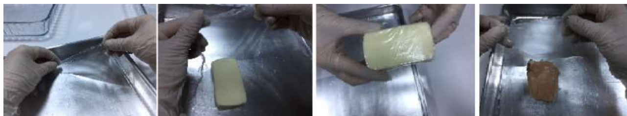
Figure 9: Film produced with PVA only
