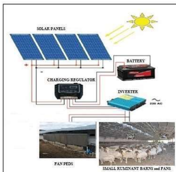
Figure 1. Components of ventilation and cooling system used in sheep folds, a type of animal house, with solar panel system
