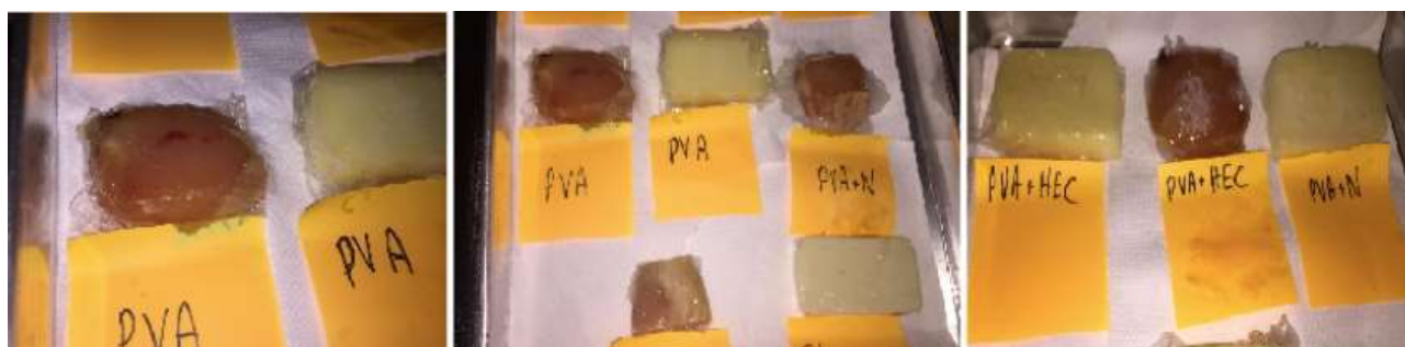
Figure 17: Testing the films with food
