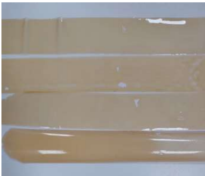
Figure 2. Adjusting the thickness of various film samples using an applicator
