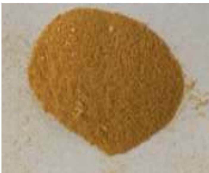
Figure 3. Film sample pulverized by cryogenic crusher
