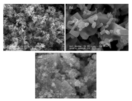
Figure 5. SEM images of (a) TiO<sub>2</sub>, (b) ZnO, and (c) SnO<sub>2</sub> nanoparticles.
