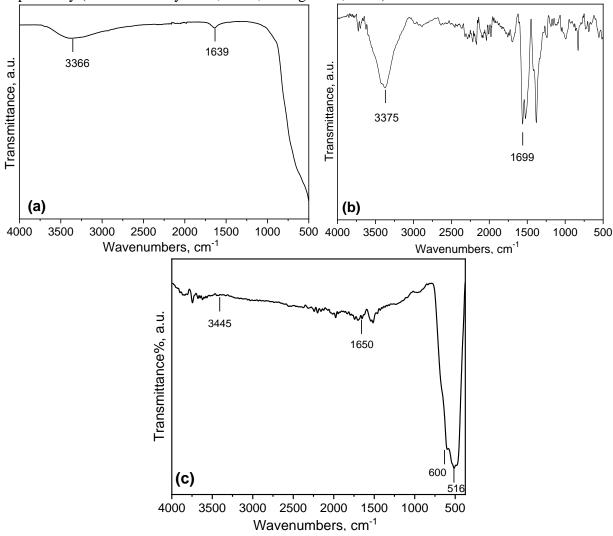
Figure 2. FTIR spectra of (a) TiO<sub>2</sub>, (b) ZnO, and (c) SnO<sub>2</sub> nanoparticles.
