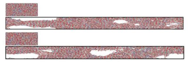
Figure 3. Atomistic images of the mPEG and mix systems after the tensile test.
