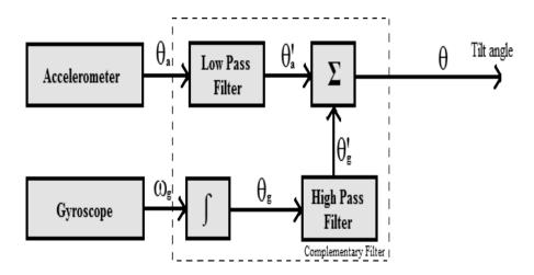
Figure 6: Flow of Complementary Filter
