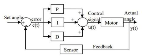
Figure 7: Closed Loop Position Control of DC Motor Using PID Controller
