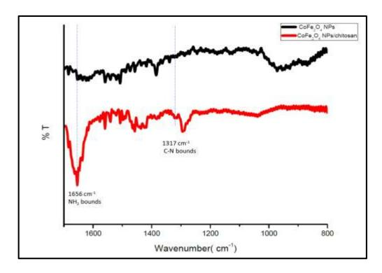
Figure 3. FTIR spectra of MNPs (CoFe<sub>2</sub>O<sub>4</sub> NPs), and chitosan-Chiotosan-MNPs
