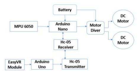
Figure 2: Block Diagram of Self Balancing Robot
