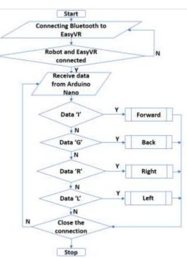
**Figure 5:** Flowchart Program From the Microcontroller
