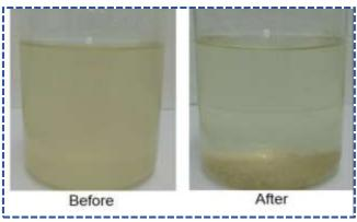
Figure 5. Flocculation process at laboratory
