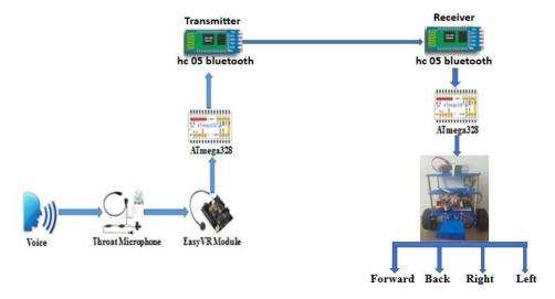
Figure 3: Voice Control General Structure of the System
