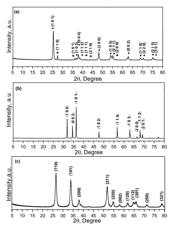
Figure 4. XRD spectra of (a) TiO<sub>2</sub>, (b) ZnO, and (c) SnO<sub>2</sub> nanoparticles.
