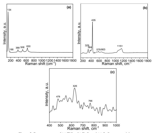
Figure 3. Raman spectra of (a) TiO<sub>2</sub>, (b) ZnO, and (c) SnO<sub>2</sub> nanoparticles.
