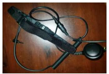
Figure 9: Throat Microphone with Two Sensors
