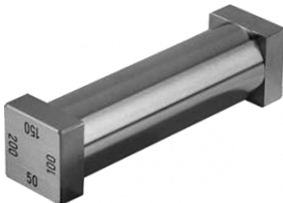
Figure 1. Applicator used to adjust film thickness
