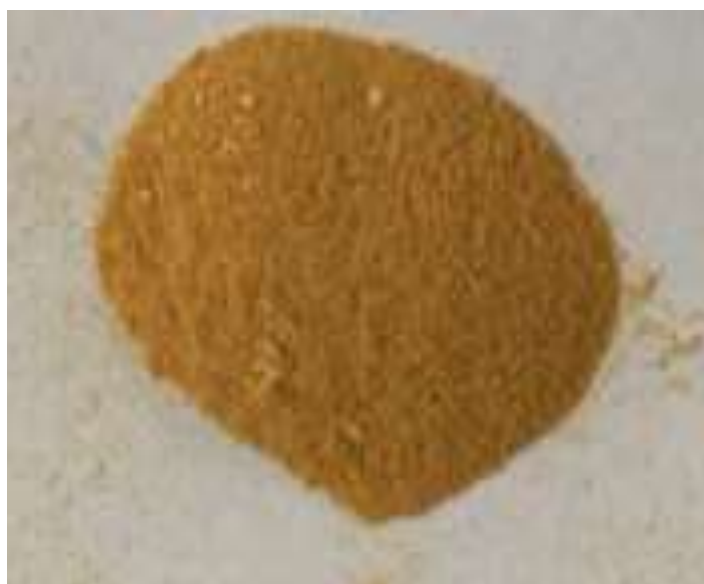
Figure 3. Film sample pulverized by cryogenic crusher
