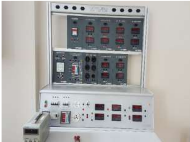
Figure 1. Electrical test set and rectifier
